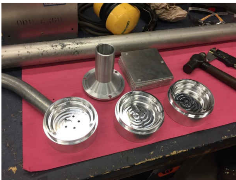
Figure 3.11. Several parts manufactured on CNC milling machine
